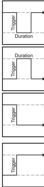
8. If you selected either **LowE** or **HighE** in the previous step, use the **Dur** knob to set the length (in frames) that the GPI output remains triggered.
