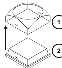
3. Place the Insert Film (2) into the Lens (1) so the readable side is facing up. The notches on the sides of the Lens must be at the sides of the text on the Insert Film.
