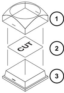
4. Aligning the notches on the sides of the Lens (1) and Diffuser (3), press the Lens and Diffuser together until they click.
