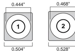
**Figure 1.9** Insert Sizing
