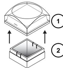
2. Remove the Lens (1) from the Diffuser (2) using a common end micro screwdriver.
