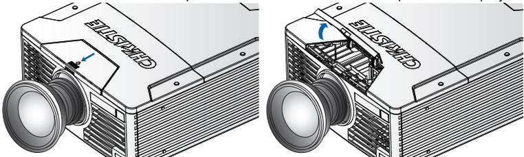
5. Push the release lever up to release the lock. Remove the lens through the front of the projector.
