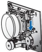
8. Lower the Lens Door and slide back into the secured position.
