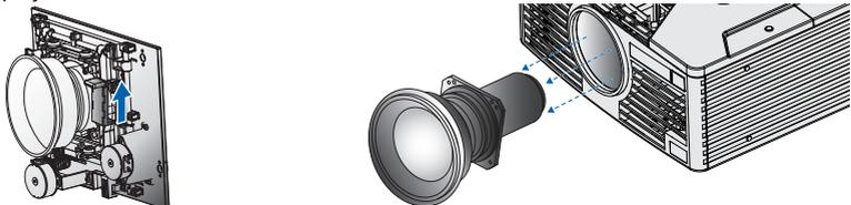
6. Remove the rear lens cap from the lens. Keep the front lens cap on the lens to protect it during installation.
