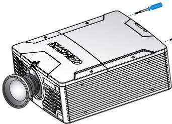
5. Open the lamp door located on the top-rear of the projector.
