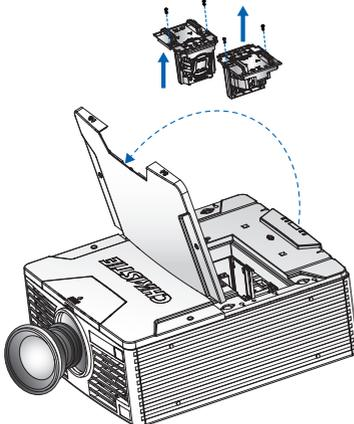
8. **Install the new lamp:** Replace the lamp with a new one and tighten two screws. Make sure the lamp is set properly and secure.
